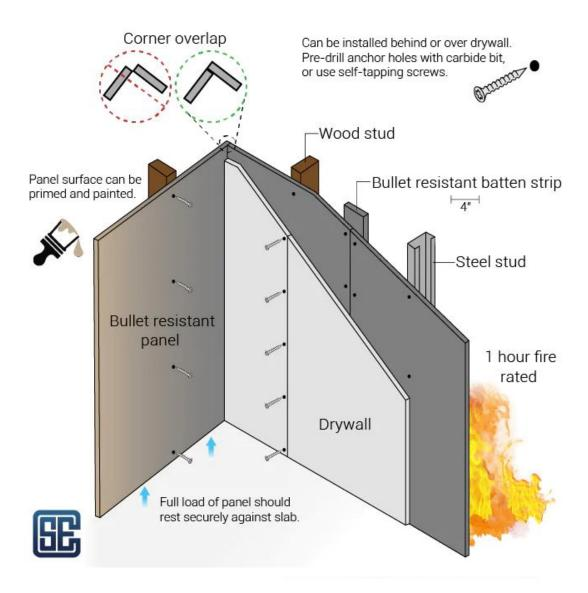
Figure 45: Armortex Installation Diagram, Accessed May 23, 2023
