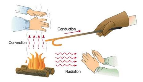
Figure 5: Diagram of Convection, Conduction, and Radiation Heat (Shirley, 2015)
