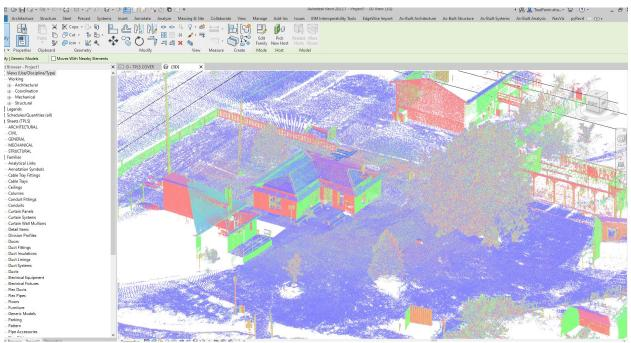
Figure 12. A point cloud file from a LiDar scan imported into Revit (an AutoDesk program utilized to create architectural and engineering 3D models and drawings of buildings).
