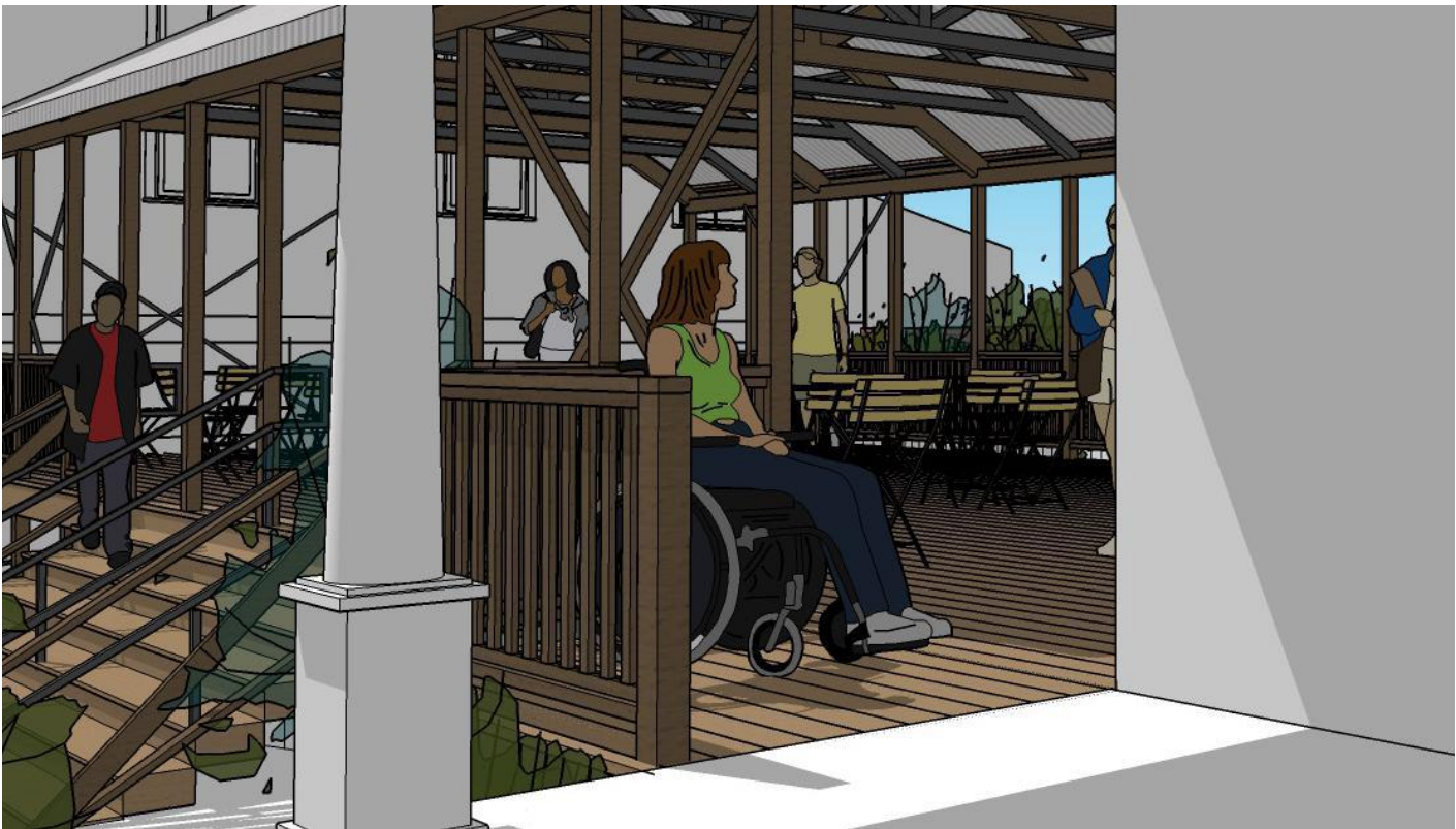
ADA platform extension: Note: fall protection at General Store via planter boxes.
