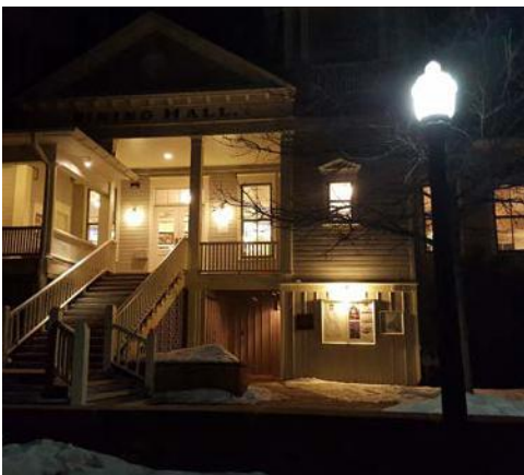
The “Acorn” style fixture in this image has potential for glare, yet the low wattage light source in it and a fairly luminous background help to balance the brightness.
