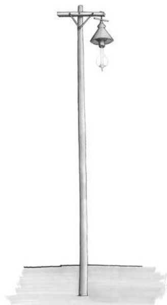
Figure 1. Sketch of original light fixture at Chautauqua. Character-defining features of the original light fixtures include orthogonal cross beams, a cone-shaped pendant, tapered pole and unornamented design.
