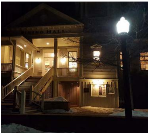
Figure G.4. The “Acorn” style fixture in this image has potential for glare, yet the low wattage light source in it and a fairly luminous background help to balance the brightness.
